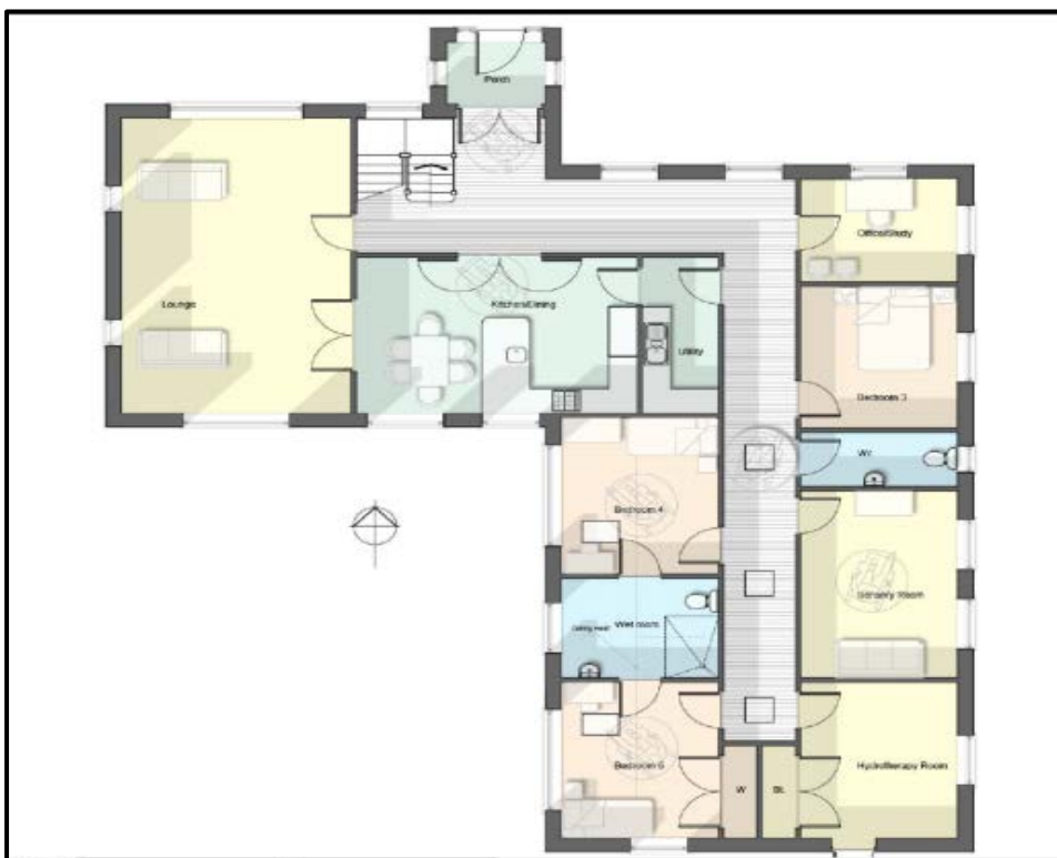
Figure 6 Proposed Ground Floor Plan
